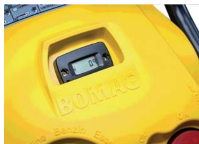
More transparency Hour meter RPM-meter with service indicator
