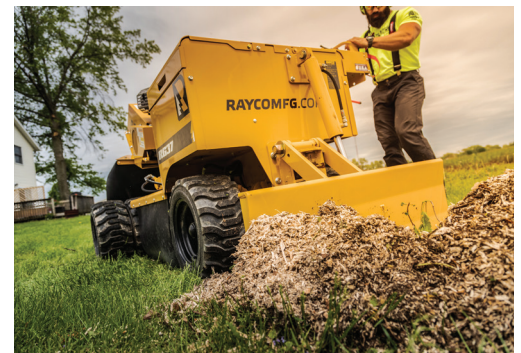
Hydraulic backfill blade for quick and easy clean up.
