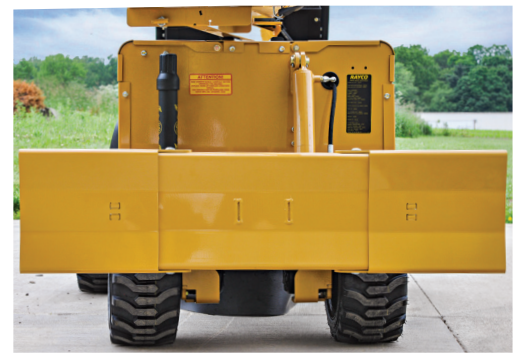
The wide hydraulic backfill blade saves time during clean up and can easily be folded in for passing through gates.
